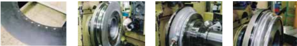
Lathe spinning of the outer stainless rim. The stainless steel will increase in strength during forming, offering interesting potential for shock absorption.
