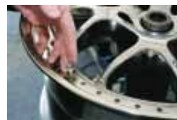
Assembly of the star hub through the stainless outer rim onto the inner rim.
