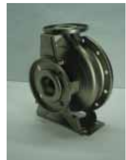
Stainless steel casing involving deep drawing
