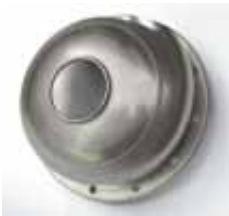
Pump casing made from a deep drawn stainless steel blank. The inlet is located on the front and the fluid leaves the casing through a hydroformed orifice at the top.
